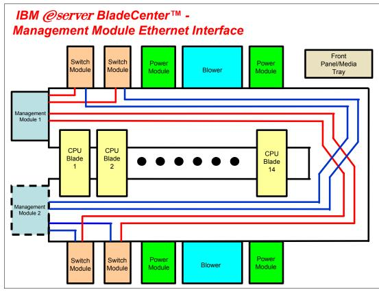
Figure 2-4 Management Module Ethernet interface
